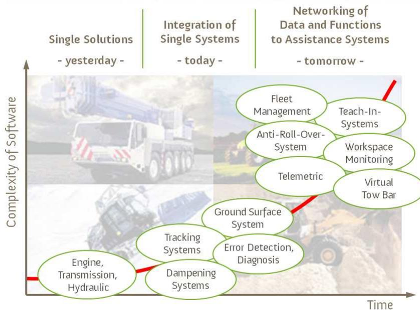
Figure 1: *Development of electronic systems in mobile machines*
